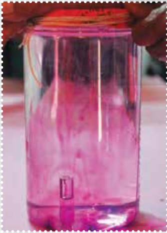
Fig. 3: Pressing the membrane and the diver going down.
