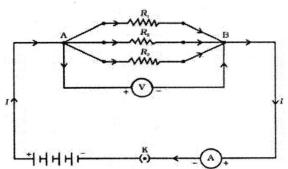
There are three resistances namely R1, R2 and R3 of value  $5\Omega,10\Omega$  and  $30\Omega$  placed in the circuit and is connected with 12 V battery as per diagram -
